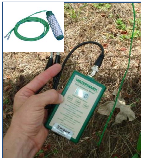
Watermark soil moisture sensor (top left) and field meter (in hand) reading “0” indicates that soil is saturated with water.
